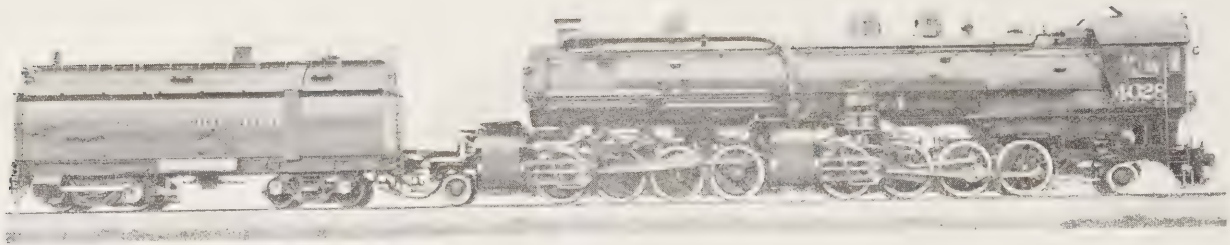
Single Expansion 2-8-8-2 Type Locomotive, Southern Pacific Lines
